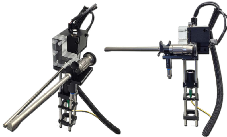
Figure 1. OCT hand piece. The OCT device mounted concurrently with a rigid laryngoscope.
