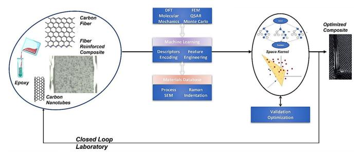
**Figure 1.** Schematic representation of a closed loop laboratory. Manufacturing, materials modelling and characterization can provide the data to correlate via data-driven AI empowered models the optimization of the next experiments in a closed-loop of information flow.
