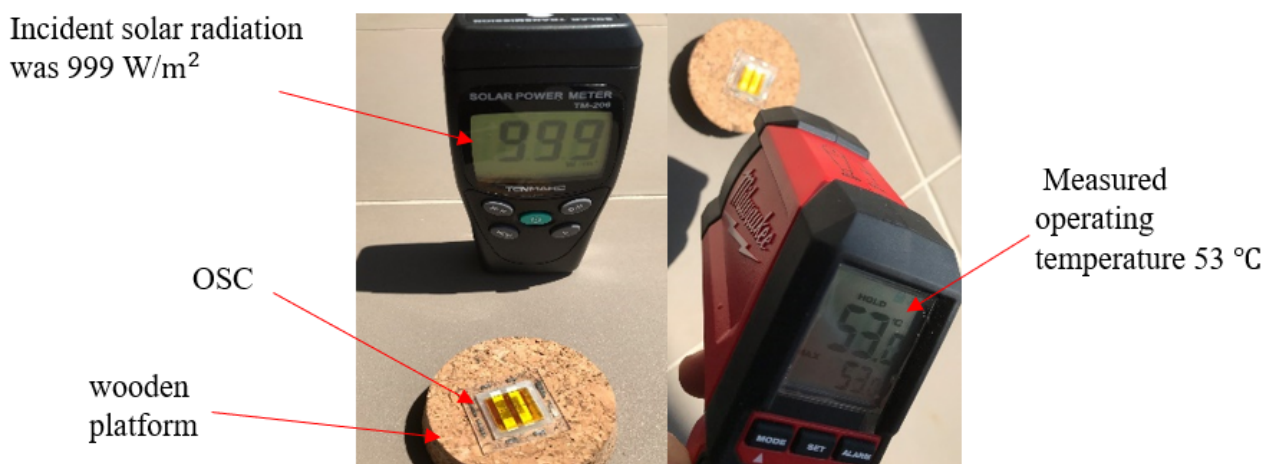
Figure 2. The measured incident solar radiation and operating temperature of the OSC in Darwin.
