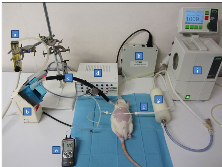
Fig. 1 Experimental setup for minimally invasive pressurized intraperitoneal drug aerosol supply in a rat placed in supine position on a 37°C heating pad; a = adjustable CO 2 flow meter; b = modified ultrasonic nebulizer (USN); c = aerosol heating tube with integrated aerosol inlet tube (40 °C); d = adjustable aerosol tube heating device; e = capnoperitoneal pressure monitor; f = aerosol outlet tube; g = high efficiency particulate air (HEPA) filter capsule; h = electronic pressure regulator device; i = aerosol evacuation pump
