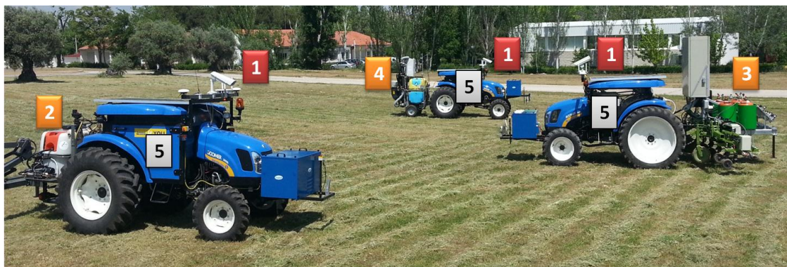
Figure 4. RHEA fleet: (1) Perception systems; (2) sprayer boom; (3) mechanical-thermal tool; (4) air-blast sprayer; and (5) unit controller.
