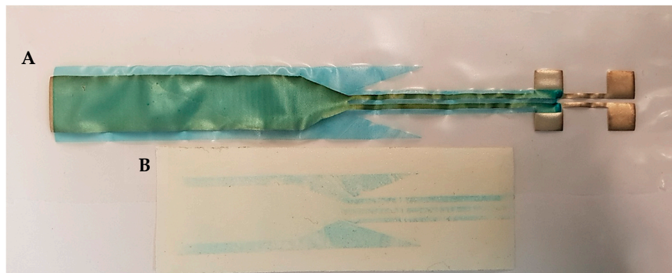
Figure 7. Peel test result. (A) The same sample after performing the peel test; (B) Tape used for the test. The blue trace indicates the poor adhesion between the substrate and the dielectric ink.
