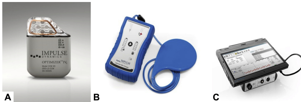
Figure 3 Cardiac contractility modulation device components: (A) Optimizer IVs active implantable pulse generator, (B) external charger used to recharge the battery of the generator on a weekly basis, and (C) device programmer (leads not shown).
