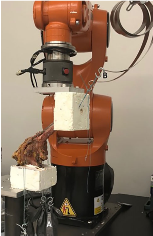
Figure 2. Robotic arm with a mounted specimen. Loading of the rotator cuff was performed using (A) deadweights (rotator cuff muscles) and (B) constant force springs (conjoint tendon and long head of the biceps tendon).
