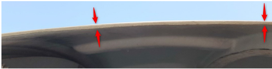
Figure 10. Unevenness of the internal surface, affecting the thickness of the dome wall.
