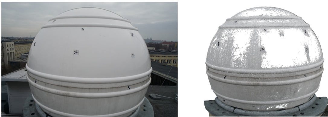
Figure 8. Comparison of the regions with pollutants and without. A photo of the dome (left) and the point cloud generated from Photoscan (right). To make the drawing easier to read, points with deviations over 25 mm have been removed from the cloud.
