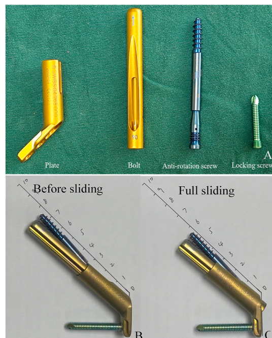
Fig. 1. A The FNS consists of (1) a threaded plate and shaft, (2) a bolt to support the proximal fragment, and (3) an anti-rotation screw. The bolt and anti-rotation screw interlock to secure the proximal fragment, and sliding through the barrel allows dynamic compression of the fracture with 20 mm of sliding space; B Before sliding, with 20 mm of sliding space; C After full sliding, shortened by 20 mm.
