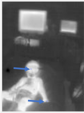
Fig. 2. An IR image taken of a patient as part of the study. Two points marked with a small cross have been selected in the image, one on the face and one on the hand of the patient to extract temperatures of corresponding locations.
