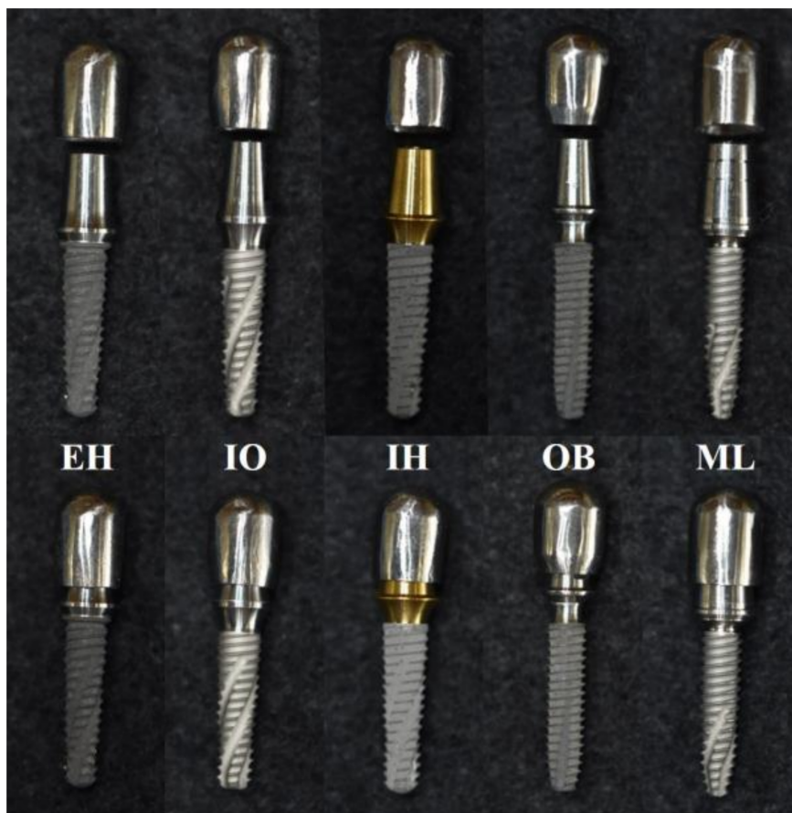
Figure 2. Examined implant systems (implants, abutments, and cobalt–chromium copings). EH: external-hexagon connection; IO: internal-octagon connection; IH: internal-hexagon connection; OB: one-body implant; ML: micro-locking implant system.
