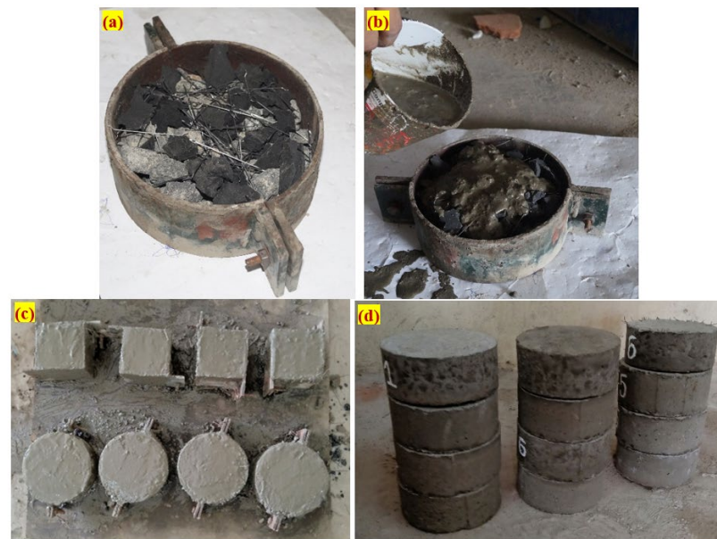
Figure 3. Casting process (a) Mold with filled aggregates and fibres (b) gravity method of grout injection, (c) finished specimens and (d) demolded specimens before curing.
