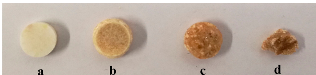
Figure 5. Physical appearance (color) for representative samples of VOR-PHP tablet compacts (a) unexposed (initial); and after storage (b) 1 d (c) 5 d (d) 10 d, at 40 °C/75% RH in open state.
