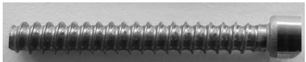
Figure 12. Forging of a screw with a ring thread of 316 LVM steel.
