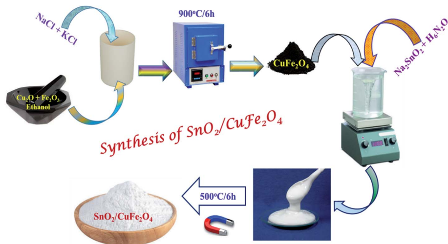
Fig. 1 Schematic diagram represents the facile route to prepare the n-SnO 2 /p-CFO complex.
