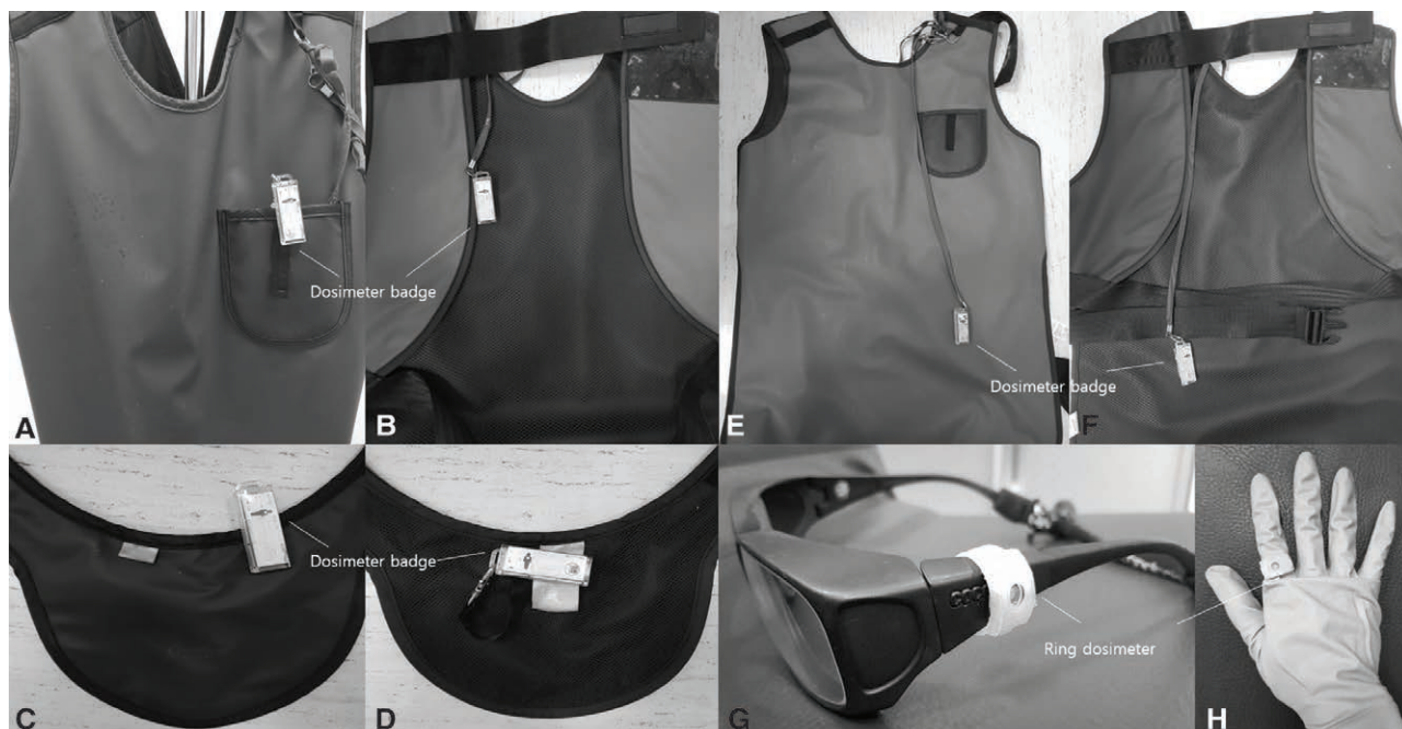
Figure 1. Allocation of dosimeters. (A) Outside the chest, (B) inside the chest, (C) outside the thyroid collar, (D) inside the thyroid collar, (E) outside the groin, (F) inside the groin, (G) on glasses, and (H) finger.
