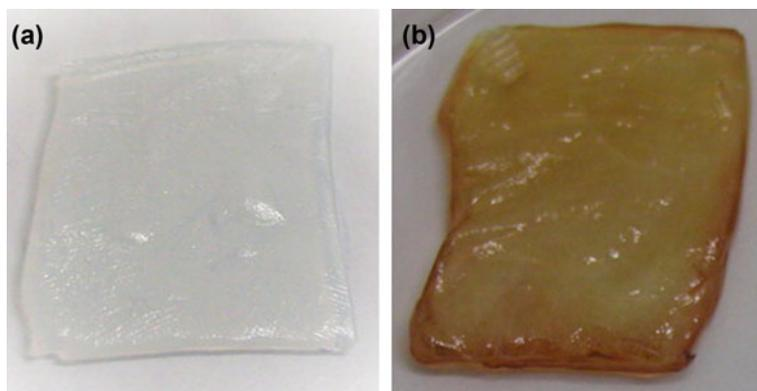
**Fig. 3** Photographic images of **a** pristine cellulose membrane and **b** Ag-cellulose nanocomposite membrane fabricated by in-situ synthesis of AgNPs. (Reproduced with permission from Pinto et al. (2009), Elsevier)
