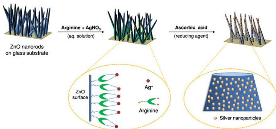
**Fig. 15** Schematic representation shows in situ synthesis and immobilization of silver nanoparticles on ZnO nanorods using arginine as a linker. (Reproduced with permission from Agnihotri et al. (2015), Royal Society of Chemistry)
