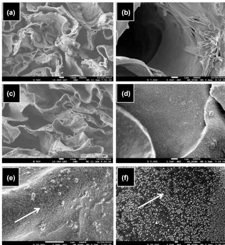
**Fig. 10** FEG-SEM images of pure chitosan-PVA hydrogel (CP-50) at **a** 9500, and **b** 97,000 magnification. **c-f** demonstrated Ag-loaded chitosan-PVA hydrogel at different magnifications: **c** 9500, **d** 97,000, **e** 920,000, **f** 933,000. (Reproduced with permission from Agnihotri et al. (2012), Springer)
