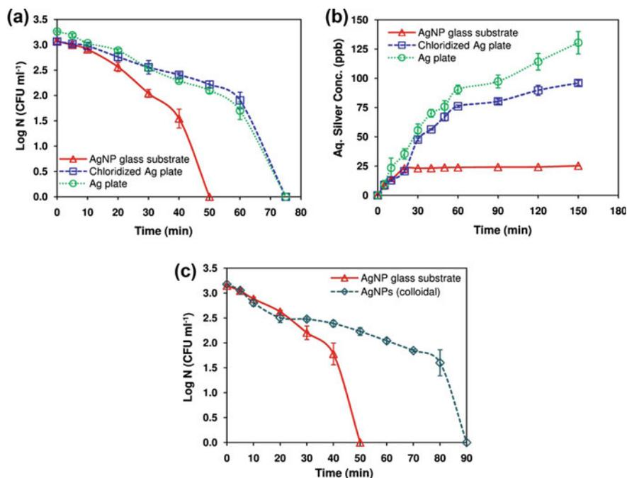
**Fig. 6** Comparative effect of various Ag sources, i.e., pure silver, AgCl and AgNP–glass substrate, all with same dimensions on **a** disinfection and **b** silver release profile is presented. **c** Comparative bactericidal potential of AgNP–glass substrate and AgNP colloidal suspension (average size 8.6 nm) against the *E. coli* MTCC 443 strain having a similar content of silver. (Reproduced with permission from Agnihotri et al. (2013), Royal Society of Chemistry)
