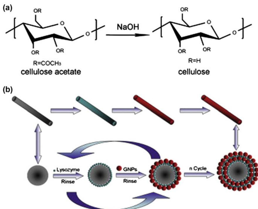
**Fig. 13** **a** Hydrolysis scheme of cellulose acetate and **b** Schematic diagram illustrating the fabrication process of the layer by layer film of GNP/lysozyme coated cellulose mats (**b**). (Reproduced with permission from Zhou et al. (2014), Elsevier)
