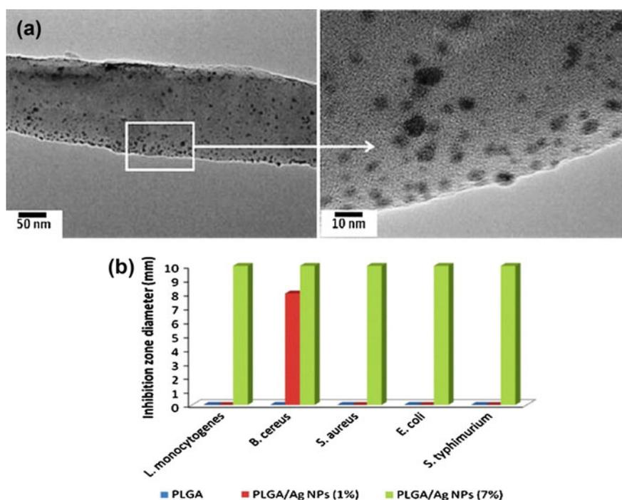
**Fig. 2** a A highly dense incorporation of silver nanoparticles on the surface of PLGA nanofibers as shown through transmission electron microscopy (TEM). b Variation in the sensitivity of microbial pathogens against silver/polymer nanocomposite as marked by difference in their zone of inhibition. (Reproduce with permission from Almajhdi et al. (2014), Springer)
