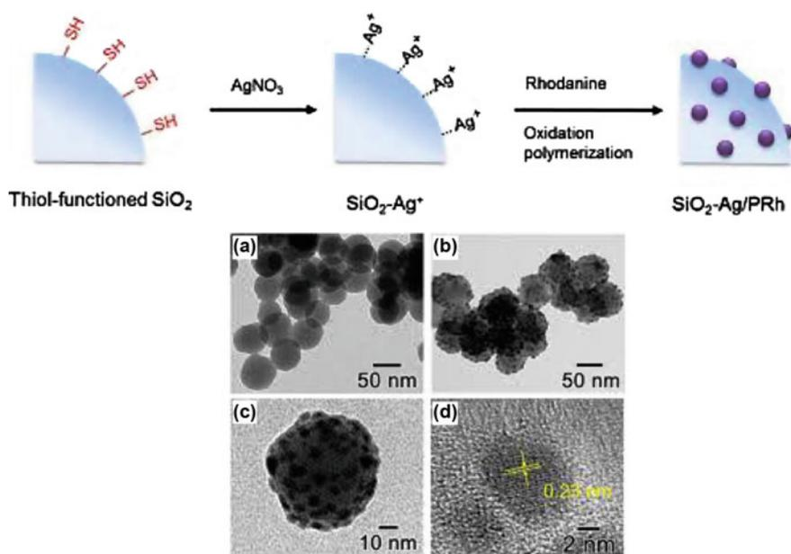
**Fig. 4** Schematic representation for the synthetic protocol of Ag/PRh-SiO<sub>2</sub> nanocomposite. TEM images of **a** thiol-modified silica nanoparticles and **b**, **c** Ag/PRh-SiO<sub>2</sub> nanoparticles at lower and higher magnifications, respectively. **d** High resolution TEM image of Ag/PRh-SiO<sub>2</sub> nanocomposite. (Reproduced with permission from Song et al. (2013), American Chemical Society)
