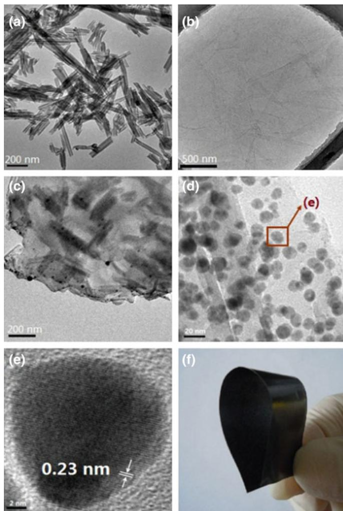
**Fig. 7** TEM images of **a** HNTs, **b** GO nanosheets and **c**, **d**, sandwich-like nanomaterials at different magnifications. **e** HRTEM image of single entity silver nanoparticles with fringe spacing. **f** Photograph of antibacterial film prepared from Ag/HNTs/reduced GO. (Reproduced with permission from Yu et al. (2014), Nature publishing group)
