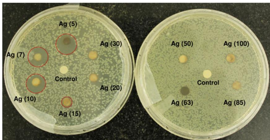
**Fig. 1** Disk diffusion tests for different sized (5–100 nm) silver nanoparticles against the *E. coli*. The zone of inhibition (ZoI) is highlighted with a dashed circle indicating a noticeable antibacterial effect. The number in parentheses indicates the average size of silver nanoparticles in nanometer (Reproduced from Agnihotri et al. (2014), Royal Society of Chemistry)
