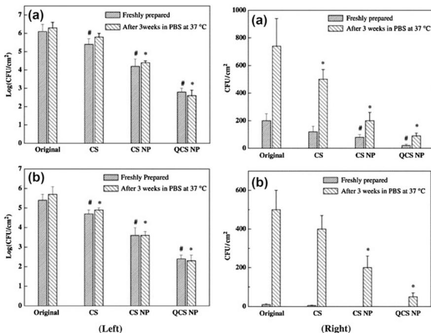
**Fig. 11** Number of viable adherent *S. aureus* (a) and *S. epidermidis* (b) cells on the different substrates based on Smart set bone cement without (Left) and with gentamicin (Right). (Reproduced with permission from Shi et al. (2006), Elsevier)
