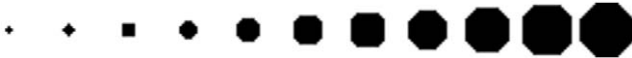
Figure 2. Structuring element. Disk of radius 1–11 pixels created using a decomposition method with a neighbourhood of 4 pixels. doi:10.1371/journal.pone.0026492.g002
