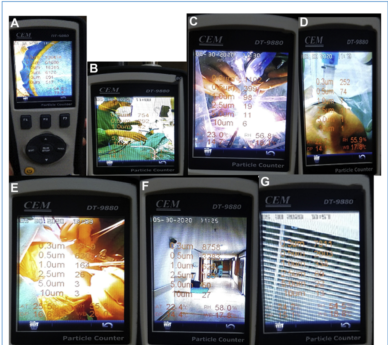
Figure 4. Particle counter recordings as seen on the CEM DT-9880 device monitor during various stages. (A) During drill use. (B) Outside the canopy
