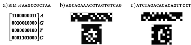
Figure 3 Image representation of a genetic sequence. a). BIM representation of AAGCCGCTAA; b). BIM (top) and image (bottom) representation of a positive training sample in data set 2; c). BIM (top) and image (bottom) representation of a negative training sample in data set 2.
