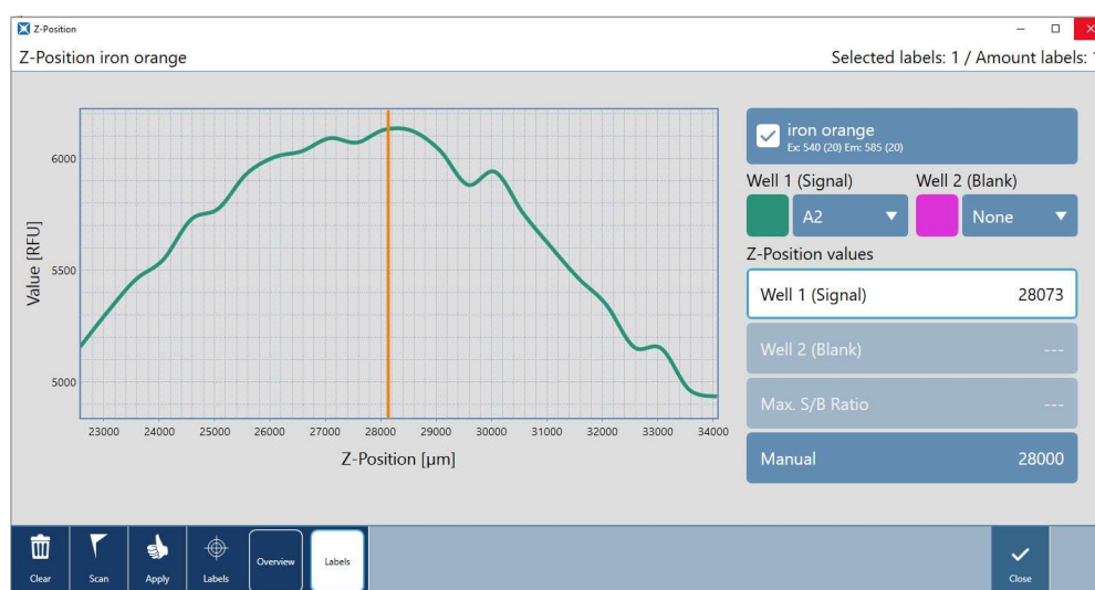
Figure 3. Screenshot of Spark plate reader calibrating the z-position. In the z-position panel of the SparkControl™ software, the user is able to measure the signal strength (x-axis) over multiple z-positions (y-axis) to determine the optimal z-position for the assay.
