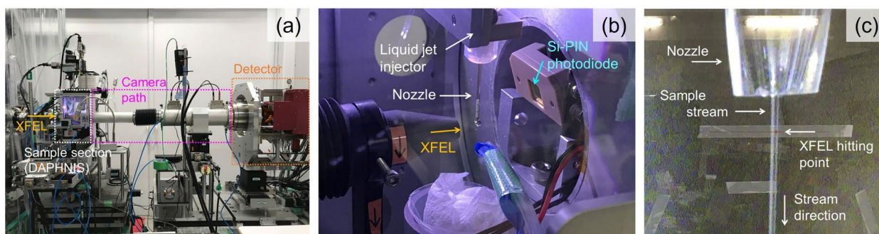
Figure 1 (a) SAXS measurement system developed for this project, illustrating the layout of the sample section, camera path, and detector. (b) Enlarged view of the sample section, highlighting the arrangement of the liquid jet injector, injector nozzle, and Si-PIN photodiode positioned on the wide-angle side directly behind the sample. (c) Close-up view of the sample stream area during the experiment, showing the injector nozzle, sample stream, XFEL hitting point, and the stream direction. The sample stream has an 83- \mu\text{m} diameter at a 1.0-mL/min pump flow rate.
