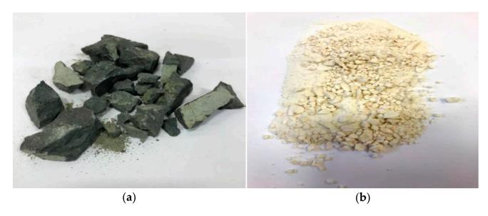
**Figure 1.** Natural raw materials from the Lower Silesia region of Poland used to melt glasses, (a) amphibolite, (b) dolomite.
