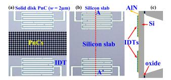
Figure 3. Micrographs of the fabricated delay lines incorporating (a) PnCs (with link width of 2  $\mu$ m) for the transmission medium and (b) solid silicon slab as the transmission medium (as the control device for comparison). (c) Transverse-view schematic of the delay line showing that the regions with IDT electrodes are released for both types of delay lines.
