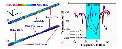
**Figure 2.** FE simulations with periodic boundary conditions applied along the y-axis—Displacement profiles of the (a) reference delay line having solid slab as the transmission medium and (b) delay line with PnCs (with inter-cell link width  $w = 3 \mu m$ ) as the transmission medium. (c) Simulated transmission  $S_{21}$  of the three delay lines showing the existence of the bandgap associated with the solid disk PnC observed through significant drops in transmission within a wide stop band.
