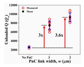
**Figure 7.** Partially covered resonators with three IDT fingers transduced in the 7th-order symmetric Lamb mode—Extracted values of unloaded  $Q(Q_u)$  of the control design with no PnCs in comparison to the two other designs with PnCs in the anchors with different inter-cell link widths. The black squares denote the mean value while the error bars denote the standard deviation over six samples for each resonator design.
