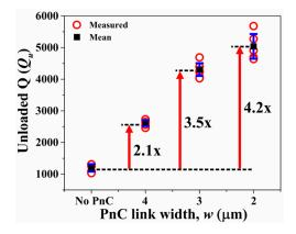
**Figure 9.** Fully covered resonators with seven IDT fingers transduced in the 7th-order symmetric Lamb mode—Extracted values of unloaded  $Q(Q_u)$  of the control design with no PnCs in comparison to the three other devices with PnCs in the anchors with different inter-cell link widths. The black squares denote the mean value while the error bars denote the standard deviation over five samples.
