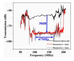
Figure 4. Measured transmission  $S_{21}$  of the three delay lines showing the existence of the bandgap associated with the solid disk PnC observed through the 30 dB drop in transmission within a wide stop band.
