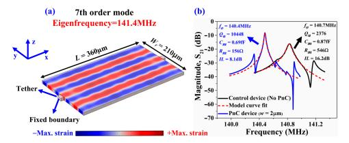
**Figure 6.** (a) FE simulation of the 7th-order symmetric Lamb mode where the contours denote the associated y-direction strain component. (b) Typical measurements of the transmission  $S_{21}$  of two of the partially covered resonators with three IDT fingers with PnC anchors ( $w = 2 \mu m$ ) and a control device (no PnC anchors) for comparison to illustrate the increase in Q; the resonators were transduced in the 7th-order symmetric Lamb mode.
