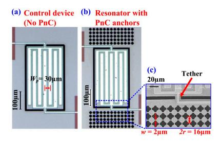
**Figure 8.** Optical micrographs of the fabricated devices: (a) Control device with no PnCs, (b) PnC bounded resonator, and (c) close-up view of the PnC matrix in relation to the Lamb mode resonator connected through the tether whose width was kept to the minimum allowed by the process.
