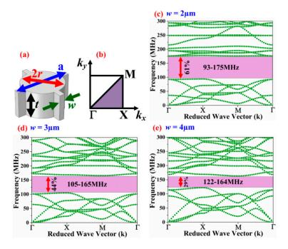
**Figure 1.** (a) Perspective view of solid disk PnC basic unit cell; (b) 1st irreducible Brillouin zone in k-space, frequency band diagrams by finite element (FE) analysis of a solid disk PnC for various inter-cell link widths of (c)  $w = 2 \mu m$  (d)  $w = 3 \mu m$  (e)  $w = 4 \mu m$ . Figures modified from the preliminary work in [25].
