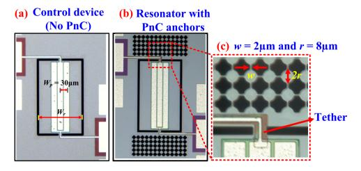
**Figure 5.** Optical micrographs of the fabricated devices partially covered with 3 IDT fingers: (a) Control device with no PnCs, (b) PnC bounded resonator, and (c) close-up view of the PnC matrix in relation to the Lamb mode resonator connected through the tether whose width was kept to the minimum allowed by the process.
