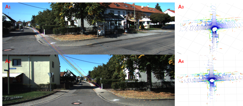
Figure 1. Complementarity between 3D point clouds and images. A_1 and A_2 are the images of the same place, which look very different since they are from two different views. A_3 and A_4 are the corresponding point clouds of images A_1 and A_2 .
