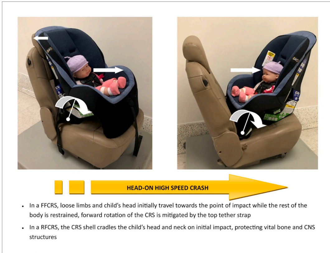
Fig. 3. Basic schematic of head-on crash mechanics pertaining to convertible CRS for forward-facing and rear-facing systems.
