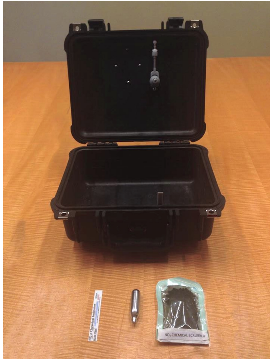
Fig 1. The Portable Sterilizer with Consumables. The portable sterilizer consists of a lockable case, a cartridge of sterilant gas, and an absorbent scrubber. A chemical indicator confirms successful sterilization.
