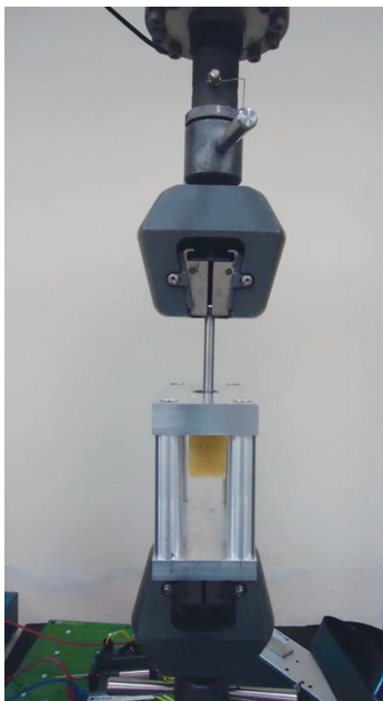
Fig. 4. Fixture frame with a test block held in the INSTRON device.
