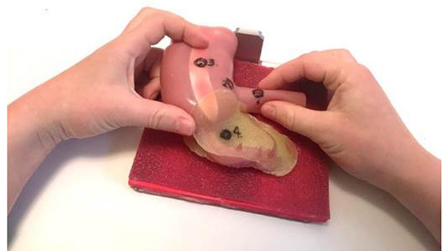
Fig. 2 Haptic exploration of the silicone ileocecal model. The circles and numbers indicate the place and the order in which a needle should be driven through the structures
