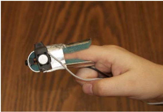
FIGURE 4. Current FingerSight device apparatus with camera and stimulator attached.
