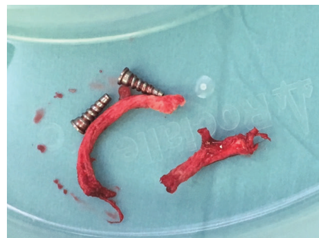
FIGURE 5: Intraoperative photograph demonstrating substantial fraying to LARS three weeks after insertion. The left fragment is the lateral limb of the LARS and the right fragment is the medial limb.
