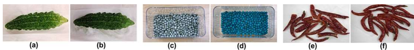
Figure 5. Comparison between the raw and dyed vegetables: (a) raw okra, (b) okra dyed with copper sulfate, (c) raw peas, (d) peas dyed with malachite green, (e) raw red chilies, and (f) red chilies dyed with Sudan red.
