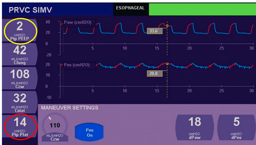
Figure 2. Esophageal and transpulmonary pressures measured in an 8-year-old morbidly obese patient with the Avea ventilator® from CareFusion. (1) Transpulmonary pressure (TPP = plateau pressure – esophageal pressure: to calculate TPP, esophageal pressure is used as a surrogate of intrapleural pressure) is 14 cmH 2 O at the end of insufflation (red circle). This means that despite a positive plateau pressure of 34 cmH 2 O in this obese child, lung parenchyma does not experience much distension (14 cmH 2 O) at the end of insufflation. (2) Positive end expiration pressure (PEEP) set on the ventilator is 2 cmH 2 O above esophageal pressure (yellow circle). This means that there is minimal risk of lung collapse at the end of expiration. Figure adapted from RM DiBlasi database with permission.
