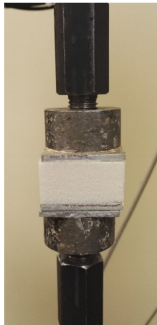
Figure 3. Cryogenic insulation rigid PU foam sample prepared for adhesion test.
