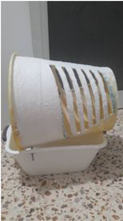
Fig. 1. The simulator structure allows to the learner to palpate ribs and to identify intercostal spaces.
