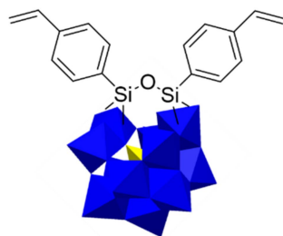
Figure 4. Structure of distyryl modified [\text{SiW}_{11}\text{O}_{39}]^{4-} via silanization. Reproduced with permission from [58]. Copyright (2019) Elsevier.
