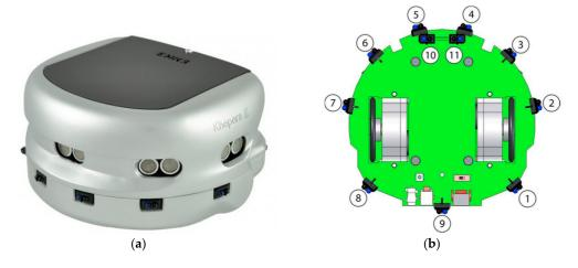
**Figure 1.** The mobile robot platform [23]: (**a**) Khepera III robot; (**b**) a bottom view of the robot showing the locations of the infrared sensor.
