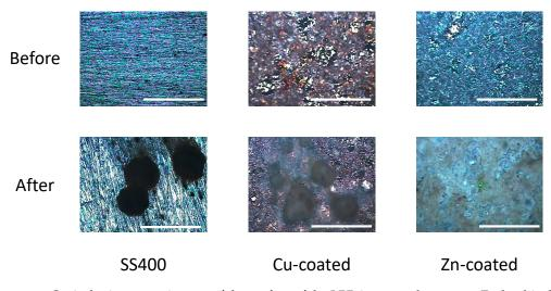
**Figure 11.** Optical microscopy images of the surface of the LBR-immerged coupons. Each white bar represents 5 mm.
