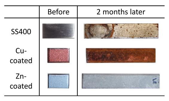
Figure 3. Digital photo images of the outdoor-exposed specimens.
