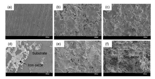
**Figure 5.** SEM images of the surface of coupons before (**a**–**c**) and after (**d**–**f**) outdoor exposure. (**a**) and (**d**) SS400; (**b**) and (**e**) Cu-coated; (**c**) and (**f**) Zn-coated.
