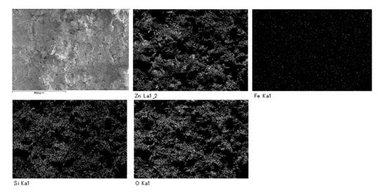
**Figure 14.** Element mapping images of the Zn-coated coupons after LBR-immersion testing exposure testing in water.
