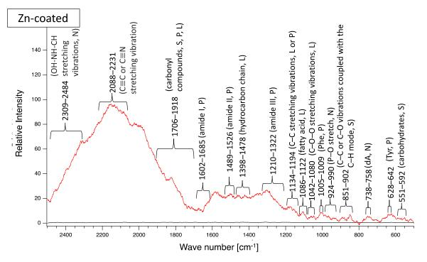
**Figure 15.** Raman peaks of sediments on the surface of the coupons after LBR immersion testing (red lines). Black lines show the Raman peaks of the surface of the specimens before the test. Detected Raman peaks after the test were assigned to related chemical bonds or compounds according to information in references [27–35]. N: nucleic acids; L: lipids; P: proteins; S: polysaccharides.
