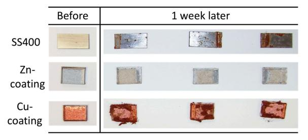
Figure 10. Digital photometric images of the surface of LBR-immerged coupons.
