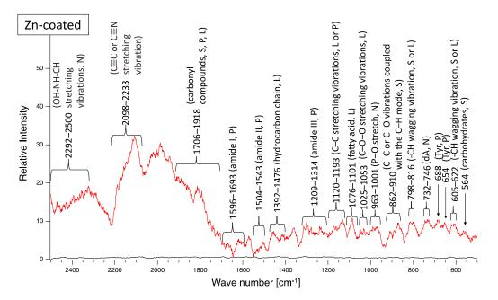
**Figure 6.** Raman peaks of sediments on the surface of the coupons following outdoor exposure testing (red line). Black lines show the Raman peaks of the surface of the specimens before the test. Detected Raman peaks after the test were assigned to related chemical bonds of compounds according to information in references [27–35]. N: nucleic acids; L: lipids; P: proteins; S: polysaccharides.
