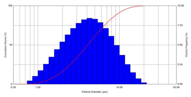
**Figure 8.** Particle size distribution of nebulized droplets of ATRA-PLGA nanoparticles aerosolized using Aerogen Solo VMN as measured by laser diffraction via Malvern Spraytec.
