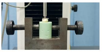
Figure 5: Showing fracture test done by compressive mode of load applied occlusally using a metallic rod with a round tip (3.6 mm diameter) using a universal testing machine
