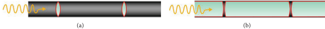
FIGURE 11: Principle of a rigid endoscope. (a) Standard rigid endoscope with high air to glass ratio. (b) Rod lens Hopkins endoscope. The reverse relation of glass to air and better coating of the lenses improves the light transmission 80-fold in comparison to the standard endoscope.
