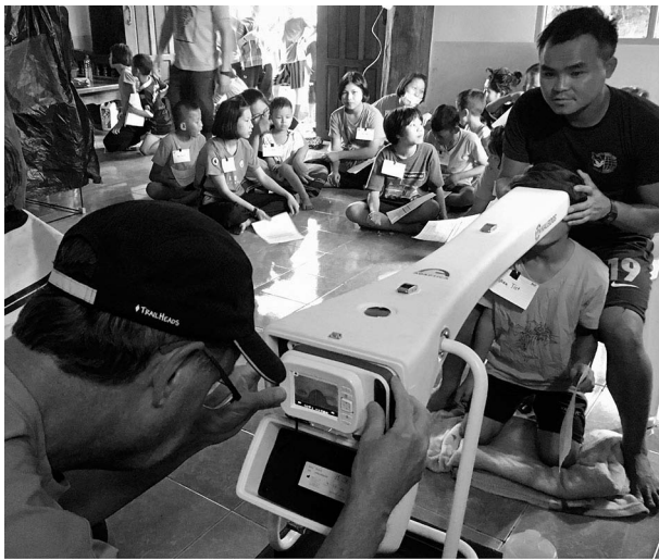
Figure 1 Kaleidos enhanced housing for 2WIN photoscreening, with housing opened to allow manual control. (Parental permission given for use of all photographs).
