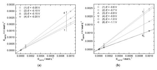
Figure 7. Langmuir isotherms for copper (a) and nickel electrodeposition (b) at different potential values.
