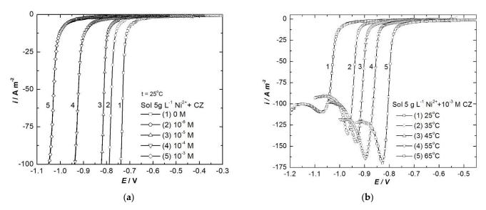
**Figure 5.** LVs recorded for nickel electrodeposition without and with different concentrations of CZ at 25 °C (a) and with  $10^{-3}$  mol L<sup>-1</sup> CZ at different temperatures (b), 2 mV s<sup>-1</sup> scan rate.
