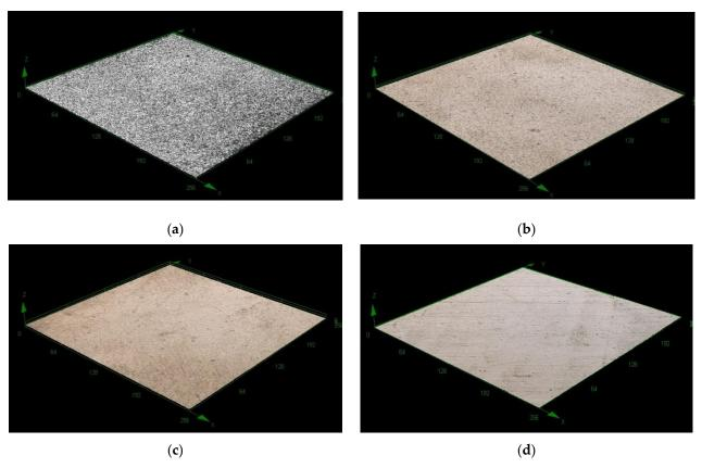
**Figure 8.** Images for copper (a,b) and nickel electrodeposition (c,d) without/with  $10^{-4}$  mol L<sup>-1</sup> CZ, magnification:  $50 \times$ .
