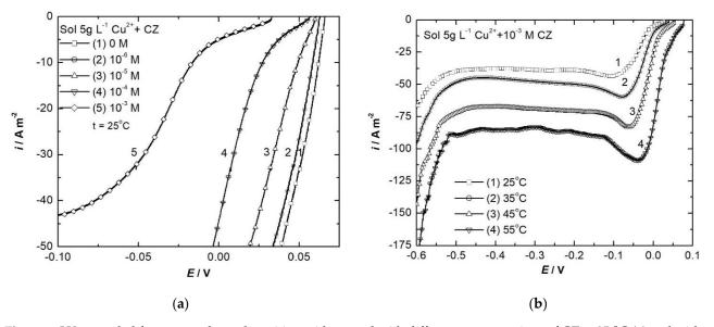
**Figure 4.** LVs recorded for copper electrodeposition without and with different concentrations of CZ at 25  $^{\circ}$ C (a) and with  $10^{-3}$  mol  $L^{-1}$  CZ at different temperatures (b), 2 mV s<sup>-1</sup> scan rate.
