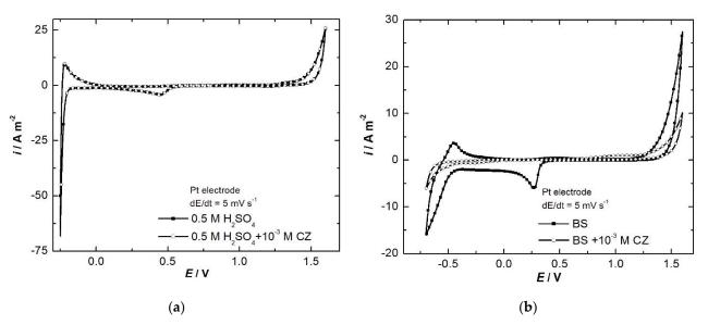
Figure 3. CVs (cycle 3) on platinum electrode  $0.5 \text{ mol } L^{-1} \text{ H}_2\text{SO}_4$  (a) and  $0.5 \text{ mol } L^{-1} \text{ Na}_2\text{SO}_4 + 30 \text{ g } L^{-1} \text{ H}_3\text{BO}_3$  (BS) (b) without and with  $10^{-3} \text{ mol } L^{-1} \text{ CZ}$ , at  $5 \text{ mV s}^{-1}$  scan rate.
