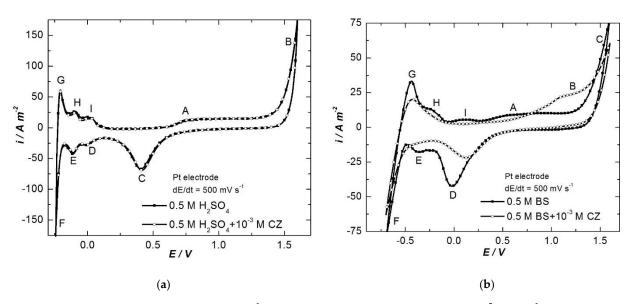
**Figure 2.** CVs on platinum electrode in 0.5 mol  $L^{-1}$   $H_2SO_4$  (a) and BS (b) without and with  $10^{-3}$  mol  $L^{-1}$  CZ, at 500 mV s<sup>-1</sup> scan rate.
