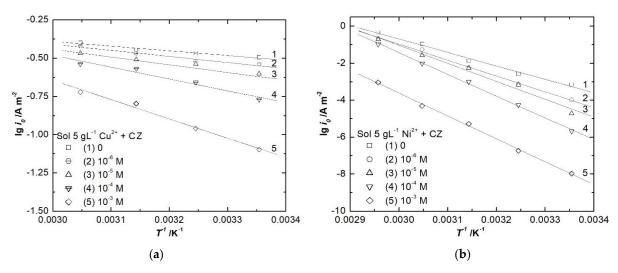
Figure 6. Arrhenius plots for copper (a) and nickel (b) deposition without and with different concentrations of CZ.
