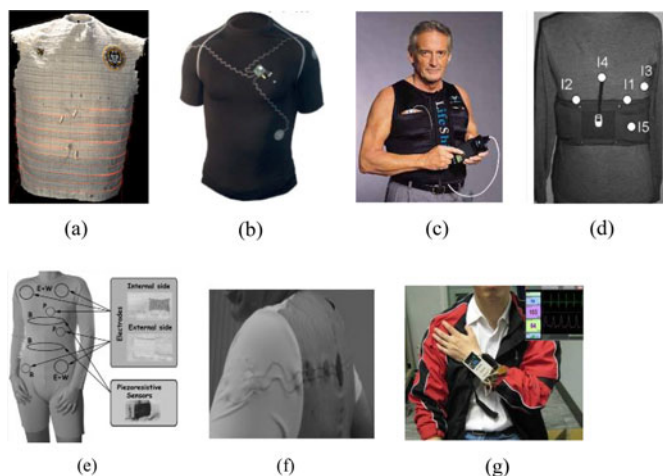
Fig. 7. Various wearable garments for physiological and activity monitoring. (a) Georgia Tech Wearable Motherboard (Smart Shirt) for the measurement of ECG, heart rate, body temperature, and respiration rate [105]; (b) the EKG Shirt system that used interconnection technology based on embroidery of conductive yarn for heart rate [106]; (c) the LifeShirt system for the measurement of ECG, heart rate, posture and activity, respiration parameters, BP (peripheral is needed), temperature, SpO 2 [107]; (d) the ProTEX garment for the measurement of heart rate, breathing rate, body temperature, SpO 2 , position, activity, and posture [108]; (e) the WEALTHY system with knitted integrated sensors for the measurement of ECG, heart rate, respiration, and activity monitoring [44]; (f) the VTAMN system for the measurement of heart rate, breathing rate, body temperature, and activity [109]; (g) the h-Shirt system for the measurement of ECG, PPG, heart rate, and BP [55].
