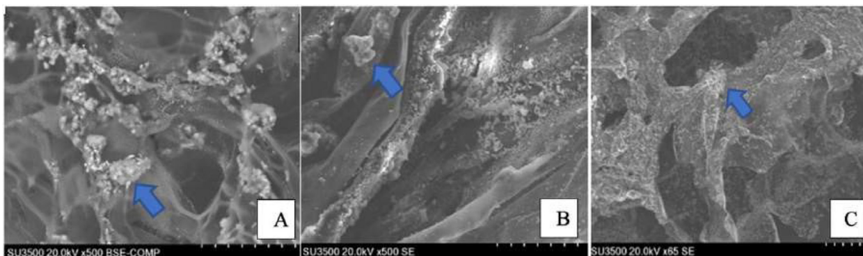
Fig. 4 HAp-Col-EGCG scaffold with 1% (A), 2% (B), and 4% (C) showed interconnected pores and agglomerated HAp dispersed in a the scaffold.
