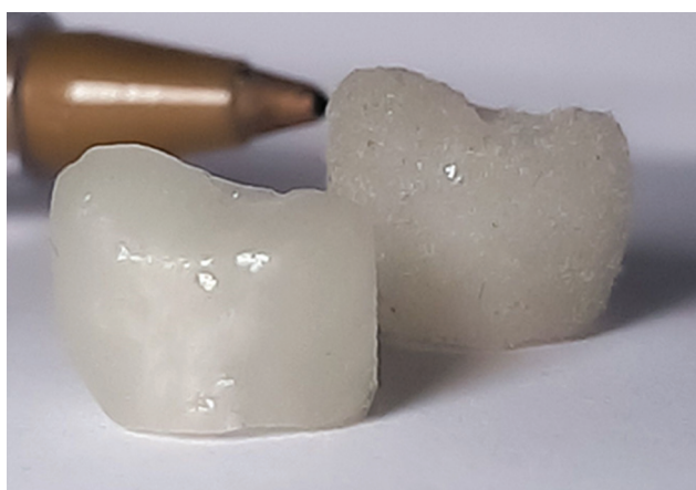
Figure 9. ZrSiO 4 -glass composite-based prosthetic crowns fabricated by indirect fused deposition modeling collapsible tool. The crown on the left side is of high grain densification with no finishing and the crown on the right side is of low grain densification with no finishing.
