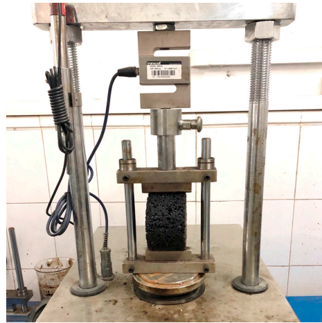
Figure 17. Loading frame used for the indirect tensile strength (ITS) test (JTG E20 T0729-2011).
