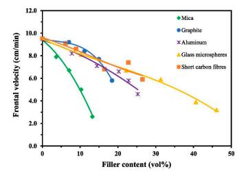
**Figure 20.** Effect of different fillers on the front velocity of a UV-cured BADGE formulation containing 1 mol % of thermal initiator TPED, 0.1 mol % photoinitiator I-Al, and 40 mol % of the diluent EOM. Reprinted from Composites Part A, 132, Anh Dung Tran, Thomas Koch, Patrick Knaack, Robert Liska, Radical-induced cationic frontal polymerization for preparation of epoxy composites, 105855, Copyright 2020 with permission from Elsevier.
