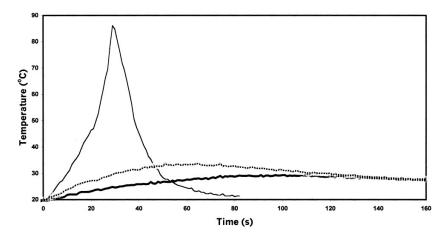
**Figure 6.** Effect of cyclohexene oxide (CHO) on the polymerization temperature and irradiation time in cationic photopolymerization of benzyl glycidyl ether (BGE). Extracted from J. V. Crivello, B. Falk, M. R. Zonca, JR., Journal of Applied Polymer Science, Vol. 92, 3303–3319, Copyright 2004 Wiley Periodicals, Inc., with permission from John Wiley and Sons.
