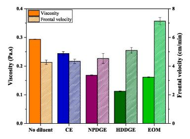
**Figure 18.** Comparison of viscosity and front velocity of several epoxy monomers in the RICFP of BADGE. Reprinted from Composites Part A, 132, Anh Dung Tran, Thomas Koch, Patrick Knaack, Robert Liska, Radical-induced cationic frontal polymerization for preparation of epoxy composites, 105855, Copyright 2020 with permission from Elsevier.
