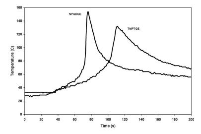
**Figure 9.** Results of the photopolymerization followed by thermal triggering for NPGDGE and TMPTGE. Extracted from James V. Crivello, Cationic photopolymerization of alkyl glycidyl ethers, Journal of Polymer Science Part A: Polymer Chemistry, 2006, 44, 3036–3052, Copyright 2006 Wiley Periodicals Inc., with permission from John Wiley and Sons.
