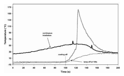
**Figure 11.** Temperature vs. time plot for frontal polymerization of glycidyl phenyl ether upon discontinuation of UV irradiation and subsequent heating after 100 s. Extracted from Effect of Temperature on the Cationic Photopolymerization of Epoxides, James V. Crivello, Journal of Macromolecular Science, Part A: Pure and Applied Chemistry, 2008, 45, 591–598, Version of record first published: 19 June 2008, reprinted by permission of Taylor & Francis Ltd., http://www.tandfonline.com.
