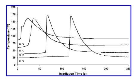
**Figure 8.** Effect of temperature on the induction time of the cationic photopolymerization of benzyl glycidyl ether. Reprinted (adapted) with permission from Umut Bulut and James V. Crivello, Investigation of the Reactivity of Epoxide Monomers in Photoinitiated Cationic Polymerization, Macromolecules, 2005, 38, 3584–3595. Copyright (2005) American Chemical Society.
