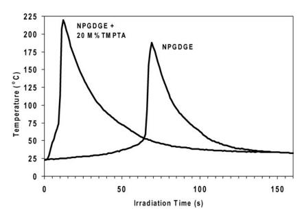
**Figure 15.** Comparison of photopolymerization of NPGDGE and multifunctional acrylate TMPTA in the presence of 2-phenyl-2,2-dimethoxy-acetophenone (DMPA) against pure NPGDGE. Extracted from James V. Crivello, Synergistic effects in hybrid free radical/cationic photopolymerizations, Journal of Polymer Science Part A: Polymer Chemistry, 2007, 45, 3759–3769, Copyright 2007 Wiley Periodicals Inc., with permission from John Wiley and Sons.
