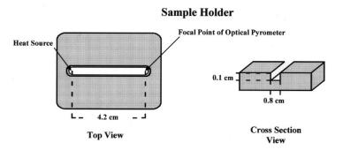
**Figure 5.** Apparatus used by Crivello et al. for studying photopolymerization of various monomers. Extracted from J. V. Crivello, B. Falk, M. R. Zonca, JR., Journal of Polymer Science Part A: Polymer Chemistry, Vol. 42, 1630–1646, Copyright 2004 Wiley Periodicals, Inc., with permission from John Wiley and Sons.
