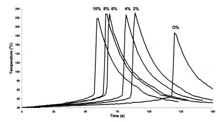
**Figure 7.** Effect of 4-vinyl-1-cyclohexene dioxide (VCHDO) on the polymerization temperature and irradiation time in cationic photopolymerization of neopentylglycol diglycidyl ether (NPGE). Extracted from J. V. Crivello, B. Falk, M. R. Zonca, JR., Journal of Applied Polymer Science, 92, 3303–3319, Copyright 2004 Wiley Periodicals, Inc., with permission from John Wiley and Sons.
