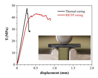
**Figure 22.** Comparison of interlaminar shear strength of thermally cured and UV-cured epoxy carbon fibre-reinforced composites. Reprinted from Composites Part A, 132, Anh Dung Tran, Thomas Koch, Patrick Knaack, Robert Liska, Radical-induced cationic frontal polymerization for preparation of epoxy composites, 105855, Copyright 2020 with permission from Elsevier.
