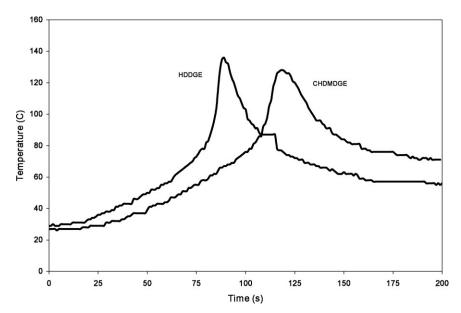
**Figure 10.** Results of photopolymerization followed by thermal triggering for HDDGE and CHDMDGE. Extracted from James V. Crivello, Cationic photopolymerization of alkyl glycidyl ethers, Journal of Polymer Science Part A: Polymer Chemistry, 2006, 44, 3036–3052, Copyright 2006 Wiley Periodicals Inc., with permission from John Wiley and Sons.
