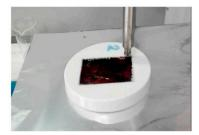
**Figure 19.** Progress of a radical-induced cationic frontal polymerization of a glass fibre-reinforced epoxy composite after 10 s of UV irradiation. Extracted from Composites Part B: Engineering, 143, M. Sangermano, A. D'Anna, C. Marro, N. Klikovits, R. Liska, UV-activated frontal polymerization of glass fibre-reinforced epoxy composites, 168–171, Copyright (2018) with permission from Elsevier.
