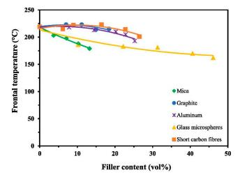
**Figure 21.** Effect of different fillers on the frontal temperature of a UV-cured BADGE formulation containing 1 mol % of thermal initiator TPED, 0.1 mol % photoinitiator I-Al, and 40 mol % of the diluent EOM. Reprinted from Composites Part A, 132, Anh Dung Tran, Thomas Koch, Patrick Knaack, Robert Liska, Radical-induced cationic frontal polymerization for preparation of epoxy composites, 105855, Copyright 2020 with permission from Elsevier.
