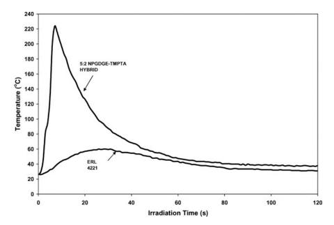
**Figure 16.** Comparison of photopolymerization of NPGDGE and multifunctional acrylate TMPTA in the presence of 2-phenyl-2,2-dimethoxy-acetophenone (DMPA) against pure ERL 4221-E. Extracted from James V. Crivello, Synergistic effects in hybrid free radical/cationic photopolymerizations, Journal of Polymer Science Part A: Polymer Chemistry, 2007, 45, 3759–3769, Copyright 2007 Wiley Periodicals Inc., with permission from John Wiley and Sons.
