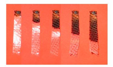
**Figure 14.** Photo-induced cationic frontal polymerization of a mixture of 5:1 TMPTGE and HDODA propagating in 10 s interval in the presence of 2-phenyl-2,2-dimethoxy-acetophenone (DMPA). Extracted from James V. Crivello, Hybrid free radical/cationic frontal photopolymerizations, Journal of Polymer Science Part A: Polymer Chemistry, 2007, 45, 4331–4340, Copyright 2007 Wiley Periodicals Inc., with permission from John Wiley and Sons.
