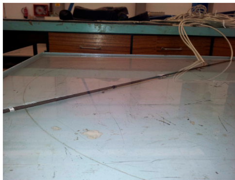
Figure 7. Sealing testing with sensors immersed in water.
